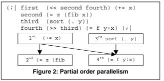
Much of DMS's parallelism can be explicitly specified based on the application of interest. However, a considerable part of DMS's parallelism is automatically extracted from DMS attribute evaluators, which are compiled into several-hundred-thousand-line partial-order parallelism PARLANSE codes. Here, DMS is acting as a code generator to produce significant parts of its own infrastructure. We believe these to be some of the largest parallel programs on the planet, and they are extremely reliable.
